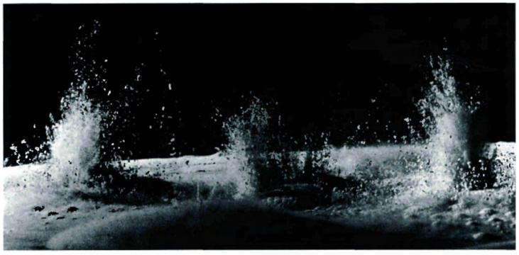
75 When the tone is loud (large amplitude) the powder is thrown up in fountains or even ejected. Yet by means of the stroboscope, which renders rapid phase sequences visible. it can be seen that vibration imposes its pattern on both the form and the dynamics of these eruptions.
