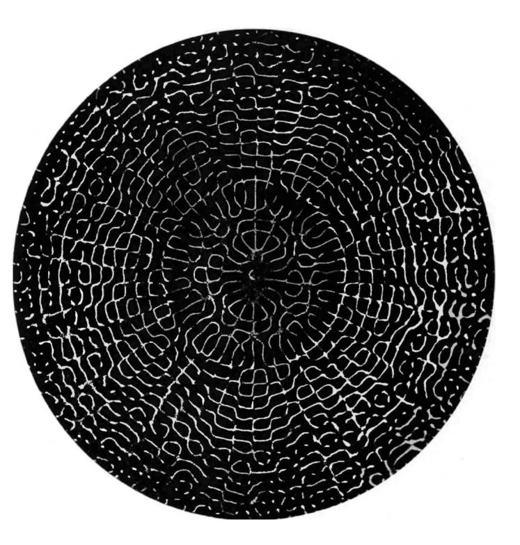
42 The same plate as figure 41 except that the frequency of vibration is 16.000 cps. By using the piezoelectric method, patterns of vibration can be produced in series. The fact that the frequency is higher than in figure 41 can be inferred by the larger number of fields.
