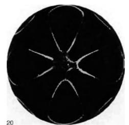
20 Sonorous figure on a circular plate. Diameter 16 cm, frequency 1060 cps. The nodal lines are made visible by sand.
