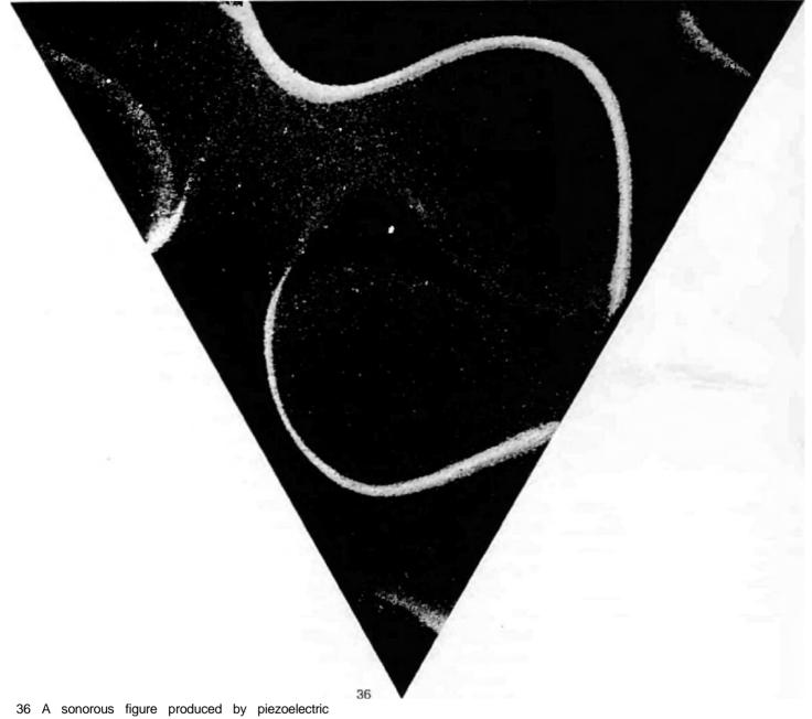
excitation. The triangle measures 24 cm along each edge. Steel plate. Frequency 875 cps.
