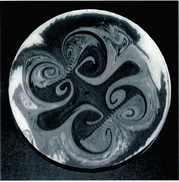
61 A stage further in the process. Several pairs of vortices have formed, each strictly bilateral in its symmetry. The vibrational field measures 28 cm across.
