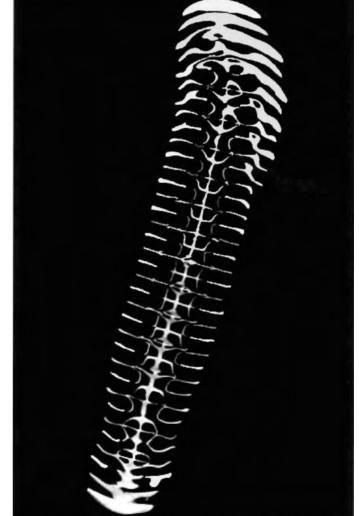
45 As in figure 44, a layer of glycerin has been made to vibrate by a tone acting upon a diaphragm. The result is a continuous formal pattern.
