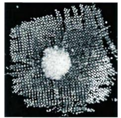
79 Under different conditions the quartz sand also forms into circulating round shapes. Fig. 79 shows a wave field of vibrating water. The sand heaps up in the center and circulates. Frequency 1060 cps.
