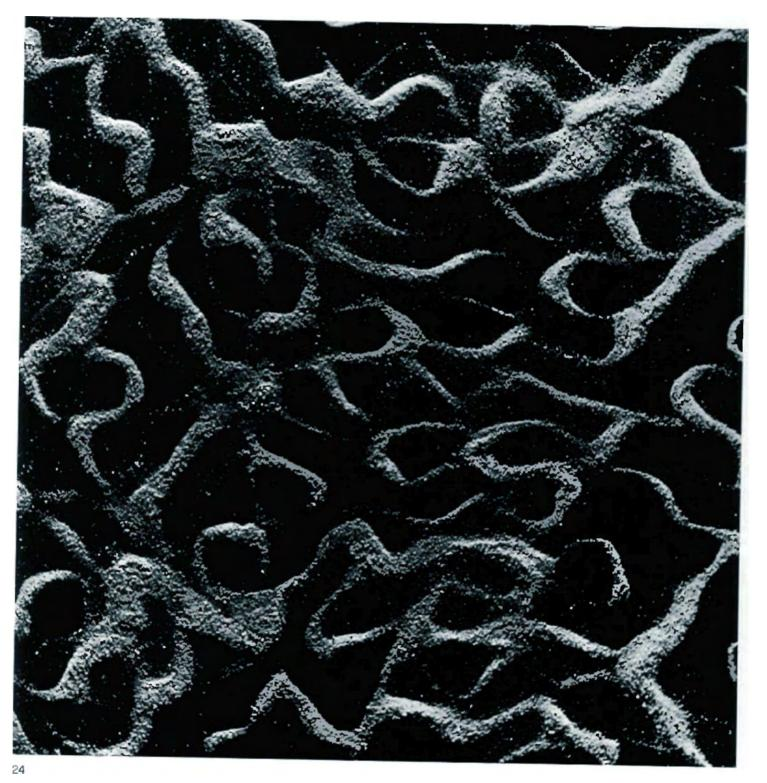
24 The sand figure is not a sonorous figure in the usual sense; the particles of sand are in a state of flow. Excitation is by crystal oscillators. Steel plate 25x33 cm, thickness 0.5 mm, frequency 10,700 cps. (Cf. figure 12.)
