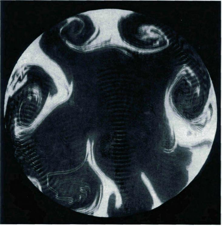
60 The process is in the nascent state, i.e. the vortices are just forming. Some wave sequences can be observed. These are a sign that vibration underlies the whole process. (Diameter 23 cm., 100 cps.)
