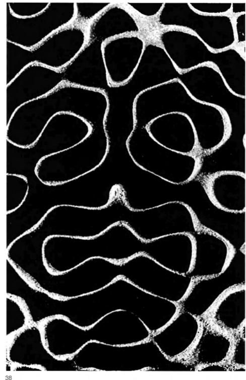
38 Sonorous figure. Plate 25 x 33 cm. Thickness 0.5 mm. 5330 cps. Configurations like these enable us to follow the variety of forms which one and the same pattern can assume. The basic pattern undergoes metamorphosis.
