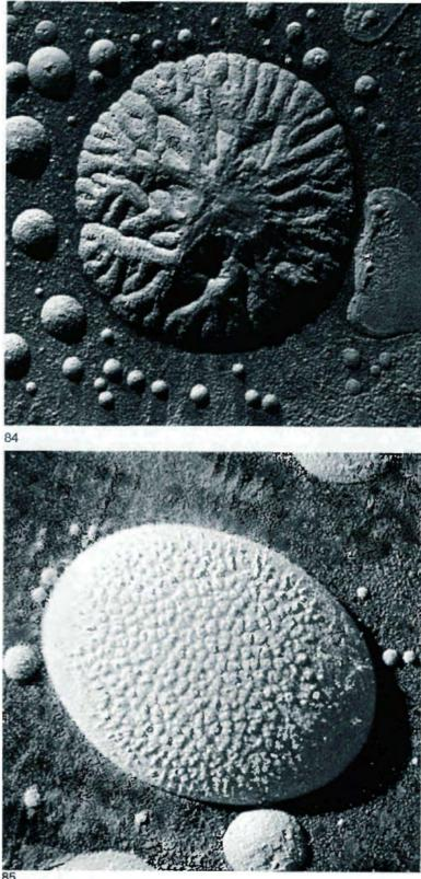
85 Again a large round form. This time the frequency was 300 cps and the pattern is accordingly of a more delicate character. (See color plate section.)
