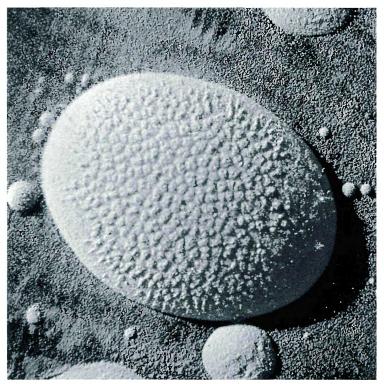
85 Acoustic irradiation transforms a uniform layer of lycopodium powder into a large round form. At a frequency of 300 cps , this more delicate configuration emerges. (See page 77.)
