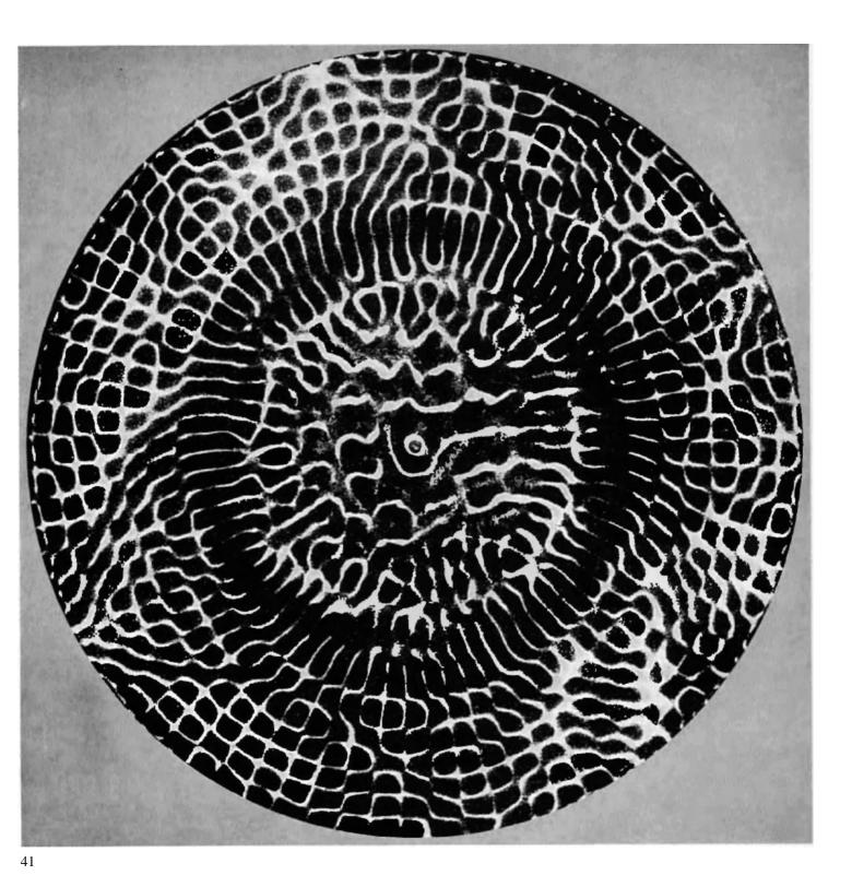
41 A sonorous figure excited on a circular steel plate. Diameter 50 cm, 6250 cps. In pictures like these the patterns resulting from radial and concentric nodal lines can be studied.
