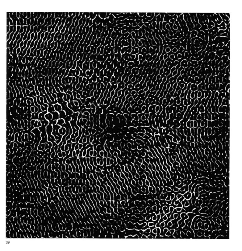
39 A sonorous figure excited by crystal oscillators. Steel plate 70x70 cm. Frequency 17,600 cps. The high frequency results in a large number of fields.
