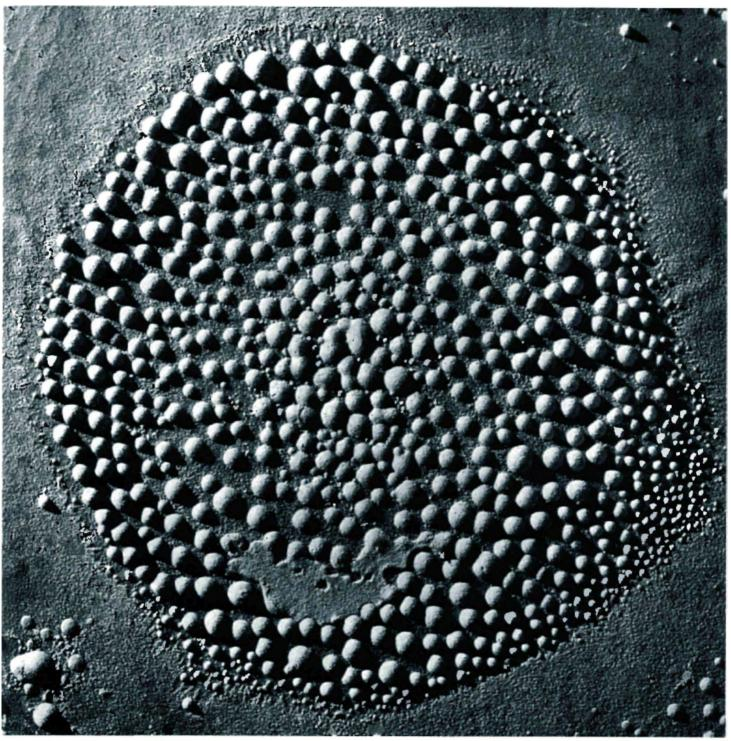
82 Acoustic irradiation transforms the uniform layer of lycopodium powder into a number of round shapes. Each of these rotates on its own axis and at the same time circulates in a constant manner around the whole figure.
