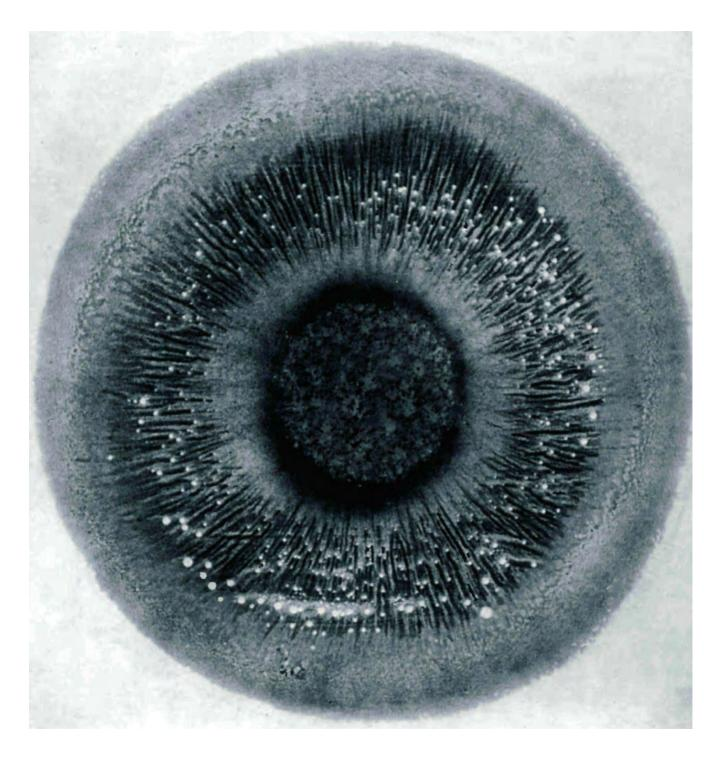
83 On a crescendo, the round heaps migrate to the center following the topography imposed by the vibration. The numerous radial pathways can be seen.
