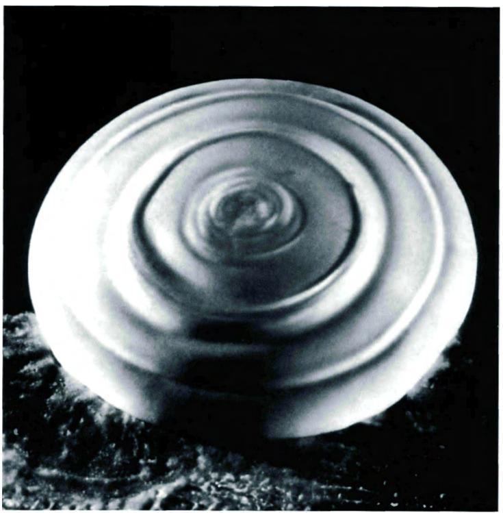
145 Round shapes appear in addition to the wave trains, all depending on the topography of the vibrating diaphragm. In figure 145, these waves trains appear in a concentric annular pattern.
