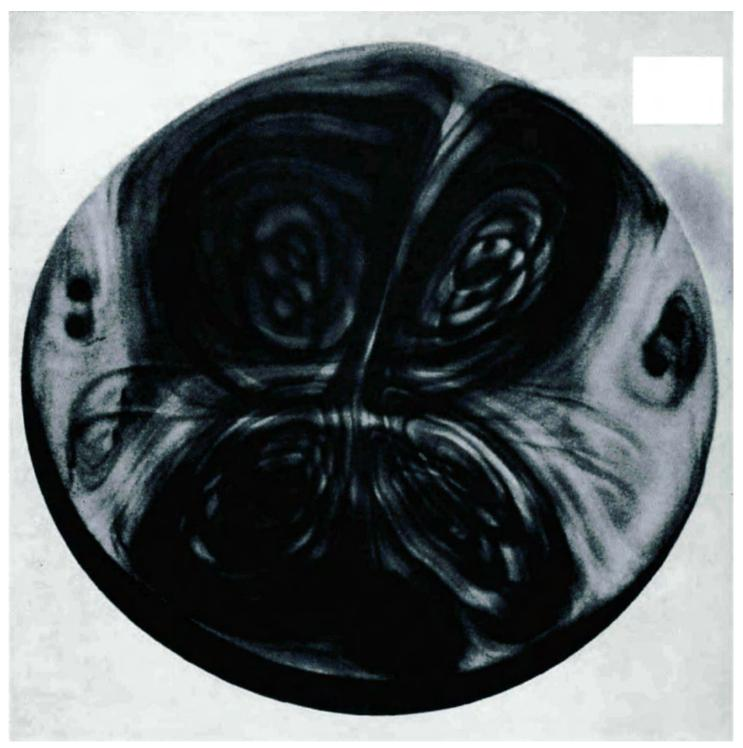
64 A pair of vortices, each pair situated in a quadrant. Again there is bilateral symmetry. The louder the tone (i.e. the greater the amplitude), the more rapid the rotation.
