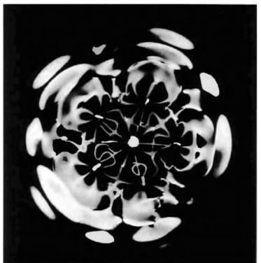
44 A layer of glycerin excited by the oscillation ot a membrane. Figures can also be seen in the liquid.
