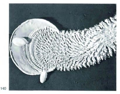
139-141 The mass has solidified. The partterns in the substance on the diaphragm are also rigid. They reflect those of the rotating round shapes (136. 137) and reveal a dendritic formation; they are not crystalline in character. (See color plate section for Fig. 140.)
