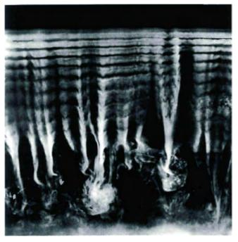
117 A downward stream of gas subjected to acoustic irradiation. The flowing veil of gas assumes a laminar patern under the influence of sound. Eddy and wave formations also appear as turbulences.
