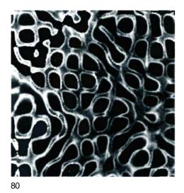
80 When conditions are different, the lycopodium powder forms sonorous figures. Figure 80 is a detail of a sonorous figure formed of lycopodium powder on a steel plate, 31 x 31 cm. Frequency 12,900 cs. This picture shows very strikingly how the powder is transported from the zones of movement towards and into the nodal zones. The precise way in which the double contours mark out the nodal zones is very conspicuous.
