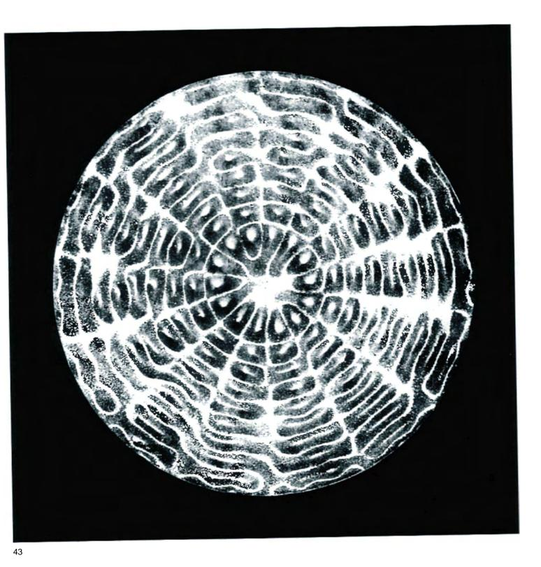
43 Sonorous figure. Plate: diameter 32 cm, thickness 0.5 mm, the material is strewn quartz sand, frequency 8200 cps.
