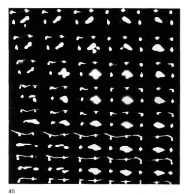
46. 47, 48 Numerous varieties of "woven" patterns are found in various materials, particularly liquids. These forms may have a cellular (46), honeycomb (47), or imbricated (48) appearance and are produced in the liquid by vibration.
